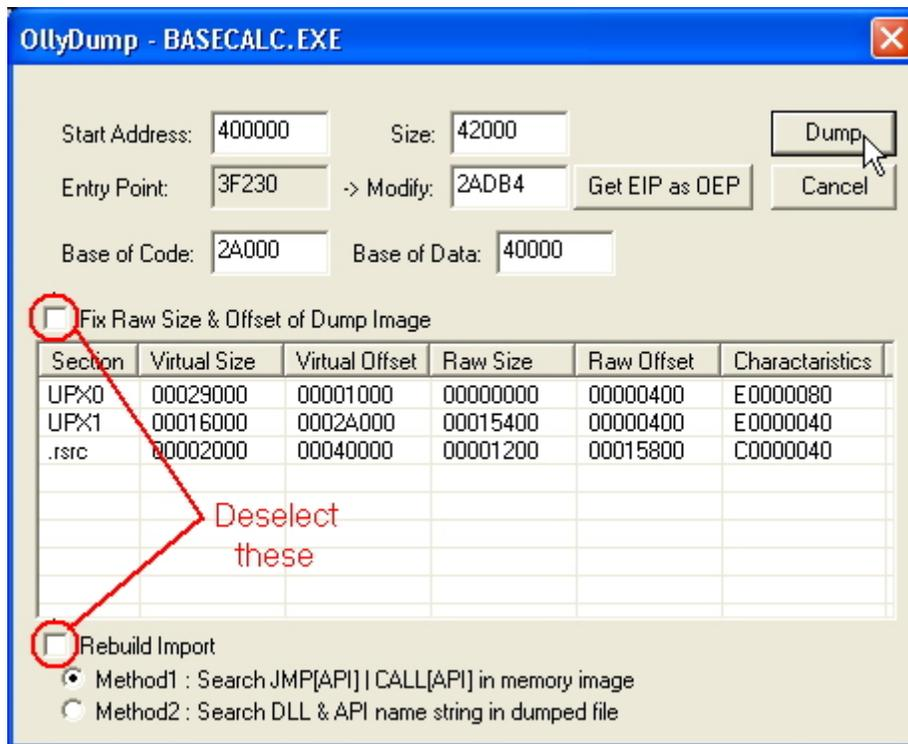
Note that OllyDump has already worked out the base address and size of image (which you could see by looking in the memory map window) and has offered to correct the entrypoint for us (although we could do
