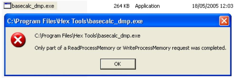
This is because of the alignment issues mentioned earlier - the filesize has also increased as a result. Open the app in LordPE and look at the sections. The raw offset and raw size values are wrong. We will have to make the Raw values equal the Virtual values for each section for the app to work. Rightclick the UPX0 section and select edit header:
