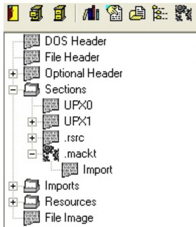
Since UPX is purely a compressor, it has simply taken the existing import data and stored it in the resource section without encrypting or damaging it. This is why ImpREC finds all valid imports without resorting to
