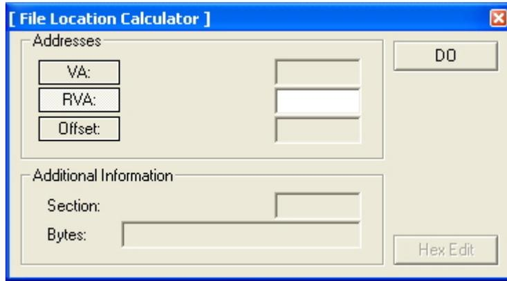
Offset Calculator also only allows conversion one-way from RVA to Raw Offset:
