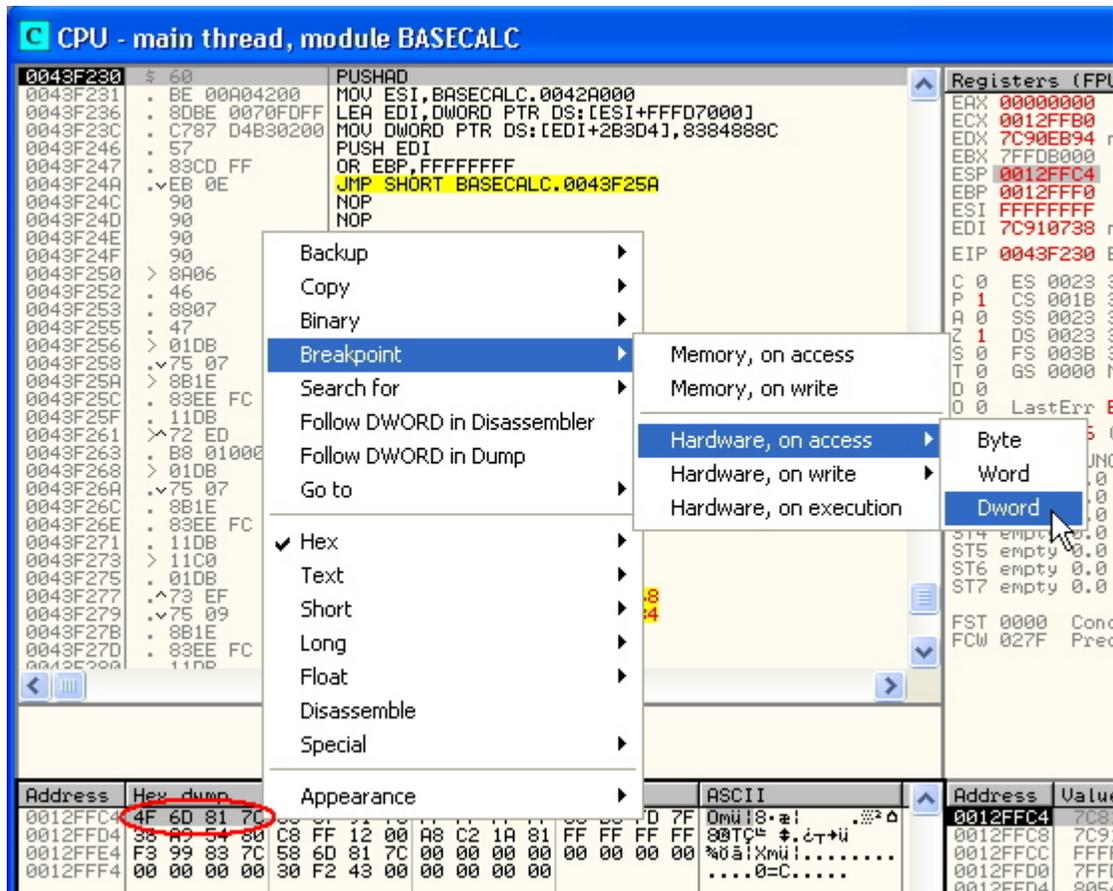
Next run the app by pressing F9 and Olly will break after the PUSHAD directly before the JMP to the OEP. The OEP shown here has the ImageBase 400000h added onto it so to make it into an RVA we subtract it which leaves 0002ADB4h:
