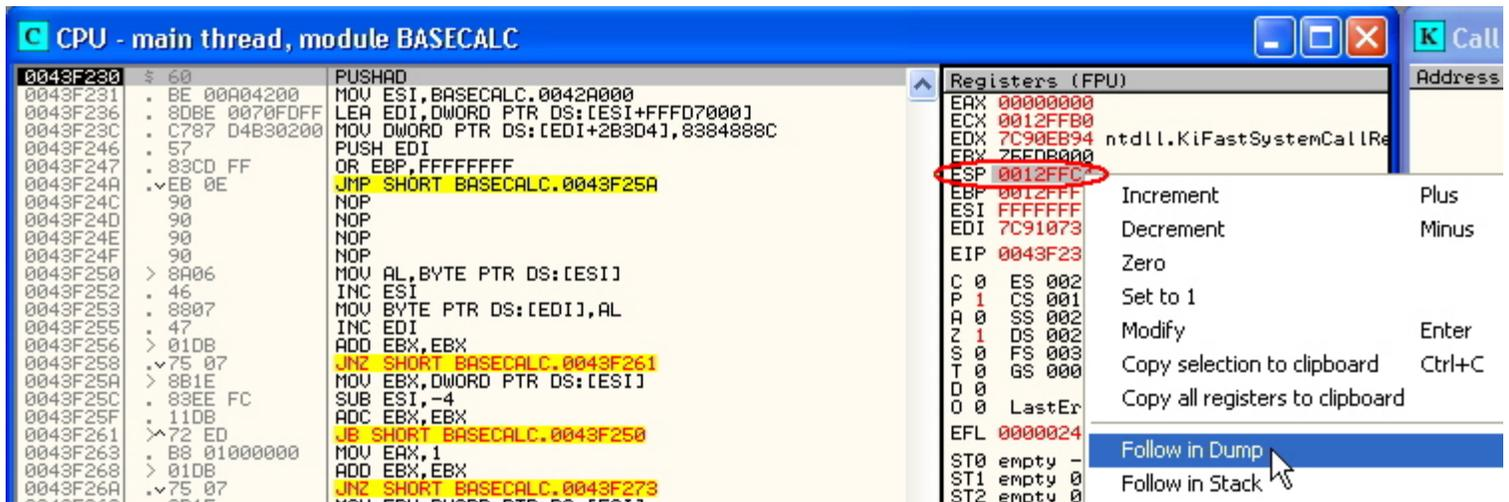
Now highlight the first DWORD of the stack, rightclick and select breakpoint, hardware on access, DWORD:
