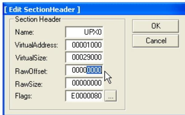
Now make RawOffset equal VirtualAddress and RawSize equal VirtualSize. Repeat for the other sections then click save and exit (this is what the "fix raw size" checkbox in OllyDump does automatically). Now the icon has returned and we get a different error when we try to run it: "The application failed to initialize properly". This is because the imports still need rebuilding.
