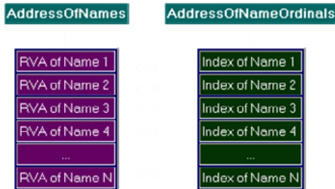
Since the EOT array exists as the linkage between the names and the addresses, it cannot contain more elements than the ENT array, i.e. each name can have one and only one associated address. The reverse is not true: an address may have several names associated with it. If there are functions with "aliases" that refer to the same address then the ENT will have more elements than the EOT.
