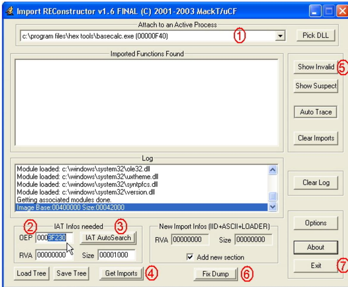
ImpREC will save a fixed copy of our dumped file appended with "\_" so run basecalc\_dmp\_.exe to test it. If we examine this file we will see that size has increased and there is an extra section called "mackt" - this is where ImpREC puts the new import data:
