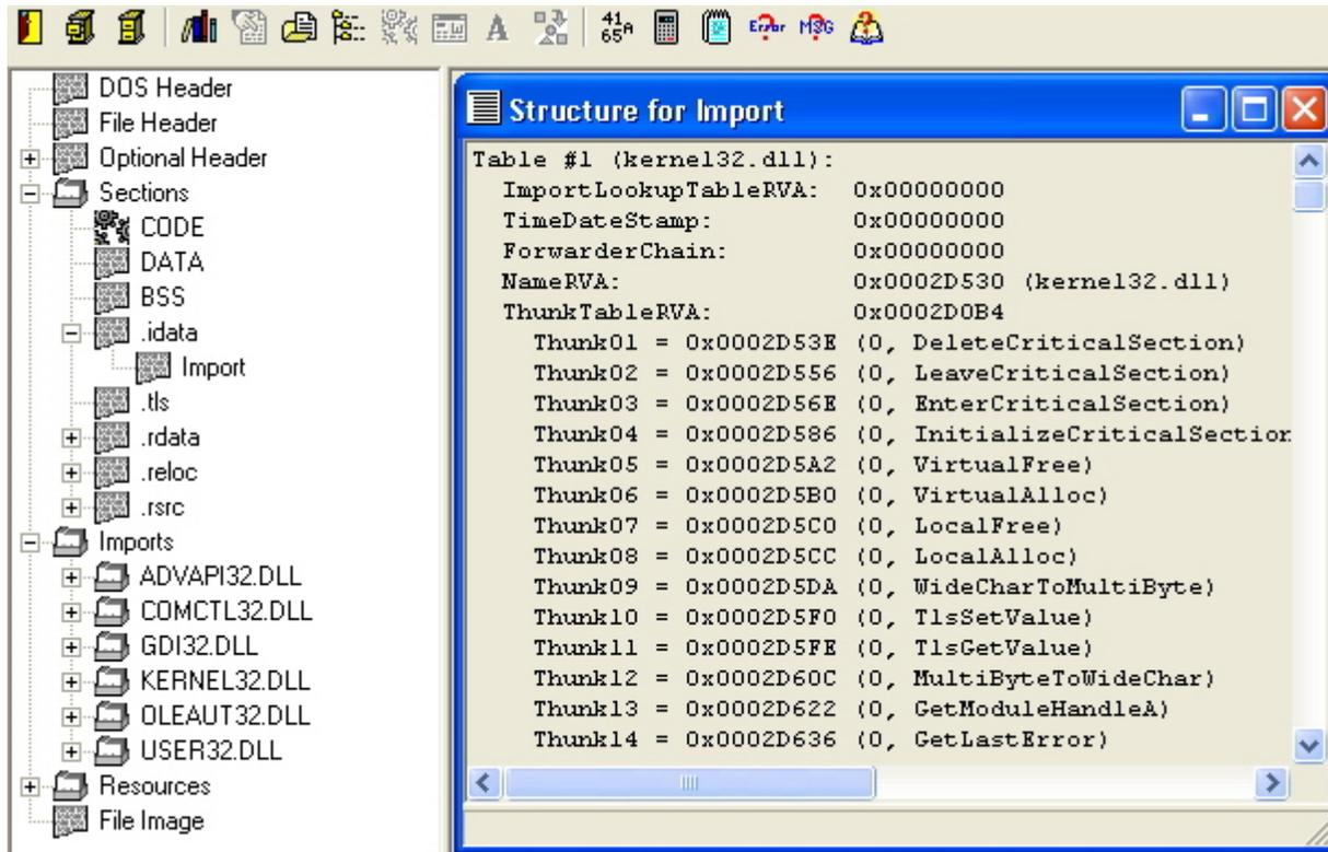
If the file had been loaded into memory, dumped and examined with the hexeditor then the DWORD at RVA 2D0B4h which contained 3E D5 02 00 on disk would have been overwritten by the loader with the address of DeleteCriticalSection in kernel32.dll:
