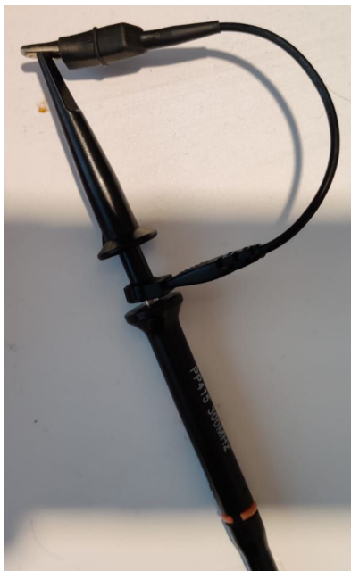
Standard oscilloscope loop shorted to its own ground, exposing a single unshielded loop
