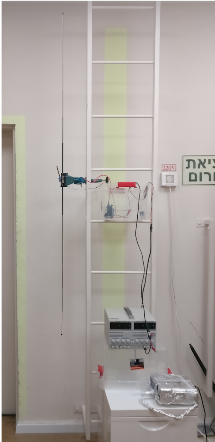
On the left: The controlled experimental setup of the EMP device. On the right: Spark gap in operation. The setup is located in an underground fortified room acting as a makeshift Faraday cage
