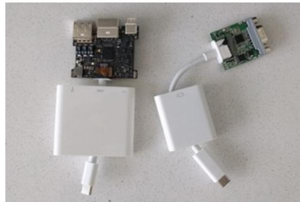
An inexpensive USB type C to HDMI adapter available for \$20 includes two programmable NXP chips for power delivery and to support the USB Billboard Device – the USB device that shows up when you plug a USB type C display adapter into a host that doesn't support display over USB type C. On this particular
