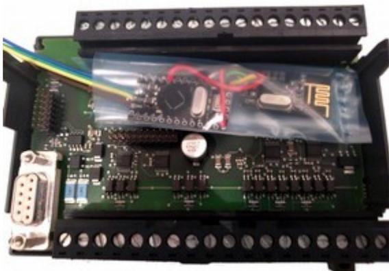
Using sample code available directly from Arduino, the implant listens for a command to set an output to high when it receives a ‘1’, low when it receives a ‘0’ and high-impedance when it receives an ‘x’.
