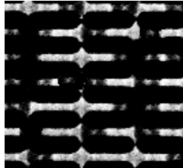
*Bits revealed by etching*
