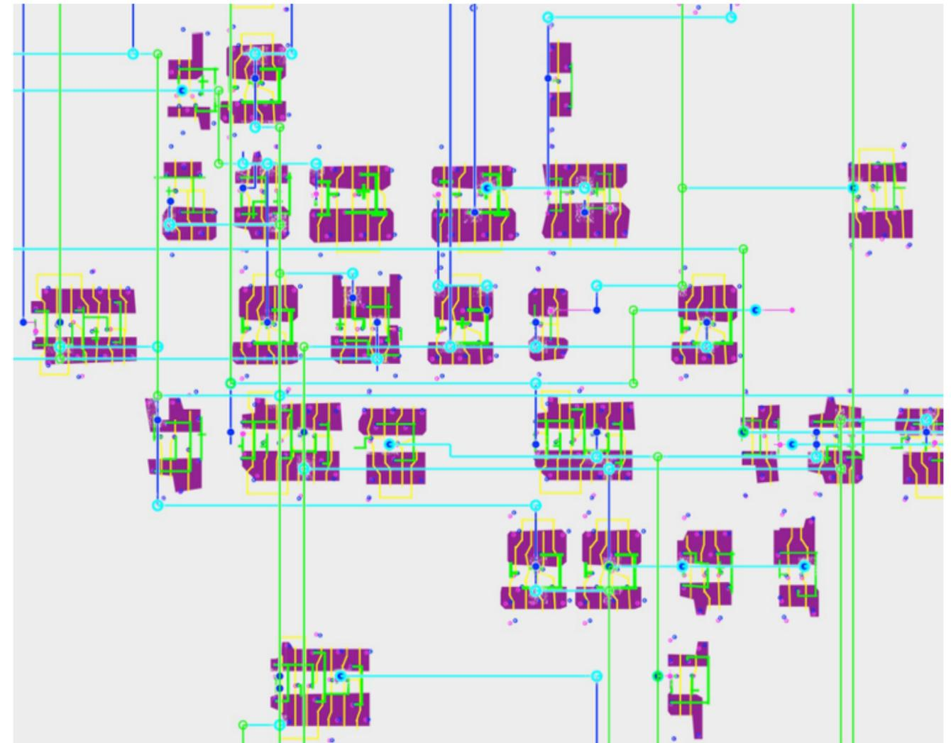
*Traced signals and their connected standard cells*
