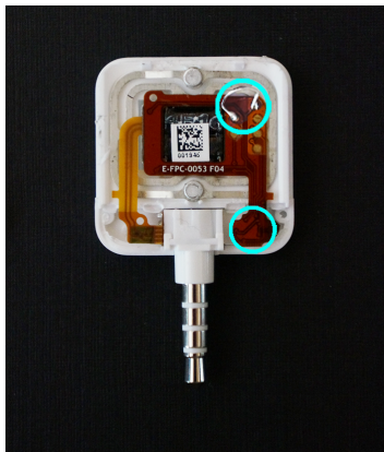
Fig. 4. The model S4 Square Reader with hardware encryption bypass implemented.
