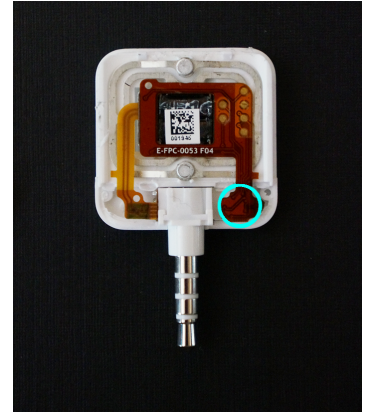
Fig. 3. The location of the model S4 Square Reader device encryption chip.
