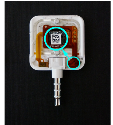
Fig. 5. In order to properly implement time-of-swipe encryption, Square should move the encryption chip to the magnetic head as shown.
