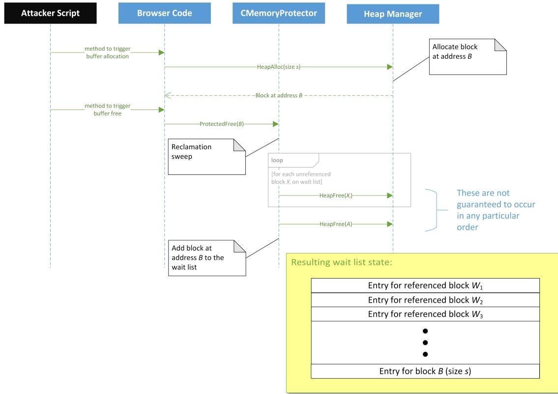
Figure 5 Sequence diagram for reclamation sweep and block add to wait list
