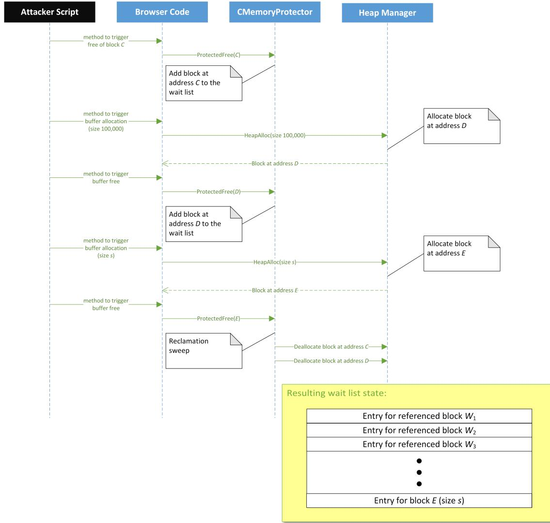
Figure 6 Diagram of strategy for clean deallocation of a block at address C
