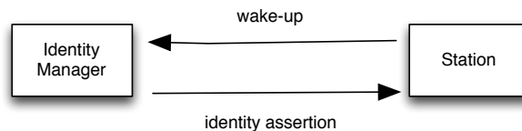
Figure 2: In the lowest security level, a proximity verification is sufficient to proceed with a transaction. The station transmits a wake-up signal that is received by the identity manager, causing it to respond with an identity assertion. The wake-up signal can contain an indicator of the station’s identity, which is compared to a whitelist kept by the identity manager. If there is a match, then an identity assertion is encrypted using a key associated with the station and the ciphertext transmitted to the station.
