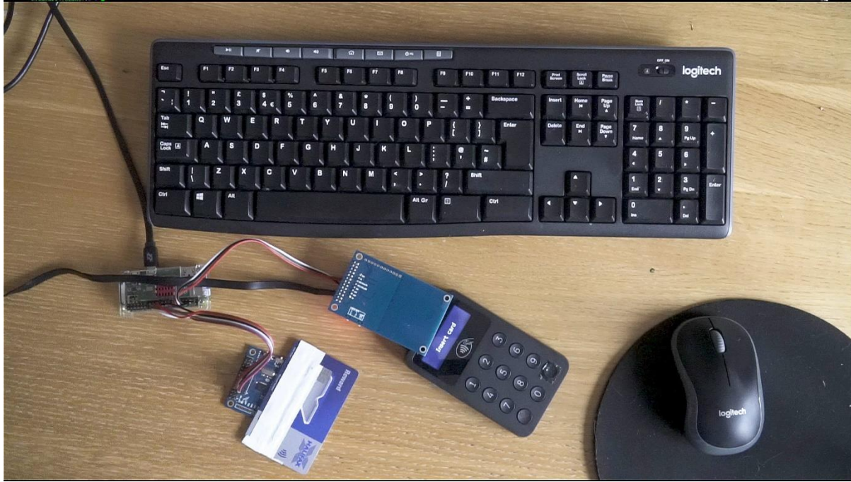
Figure 12. The terminal shows that in step six, the card does not send cardholder data and a cryptogram as expected. Instead the communication terminates and the terminal asks that the chip card be inserted instead.
