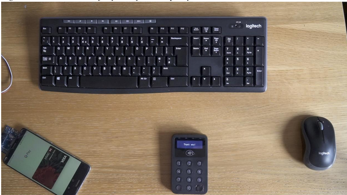
Figure 22. Payment of £31.00 successfully made without the need for the device to be unlocked
