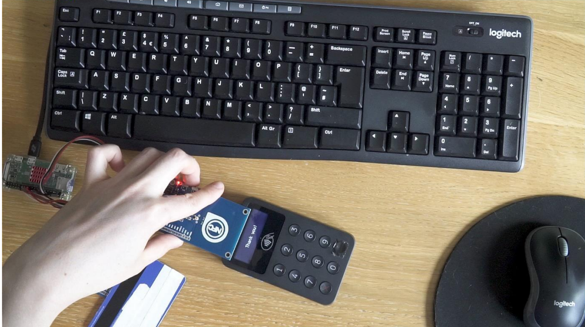
Figure 15. "CVM required" and "CDCVM performed" are substituted using the NFC proxy. Payment of £31.00 is successfully made without cardholder verification.
